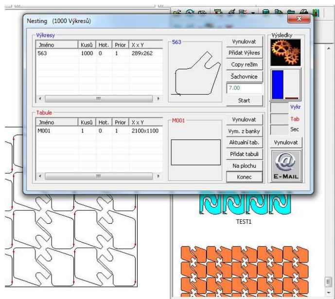
The **WRYKRYS** program also contains an internal CAD system that you can use to create your own designs or to edit loaded DXF/DWG files using the standard tools.
