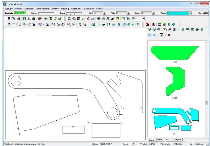
Besides communication with your internal database of designs and configurations, the sidebar also contains a large spectrum of macros (predefined shapes) including an option where you can create your own macros; also, it enables you to input DXF and DWG files and work with rests of plates to maximize utilization of your material.
